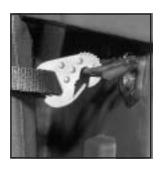
Secure the storage bag in the cargo storage area by attaching the four clips on the cargo bag to the tie-down locations on either side of the storage area.
